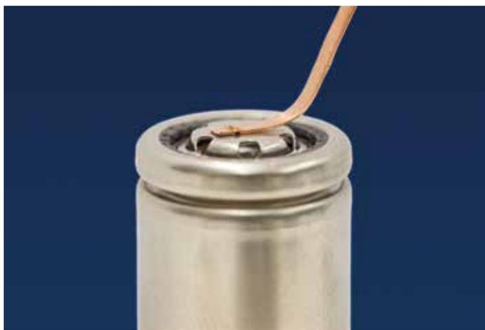
A 18650 battery cell with a laser-bonded ribbon connection. Photo: Fraunhofer ILT
