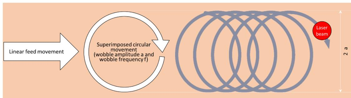
Fig. 2: Line movement in the oscillation welding procedure
